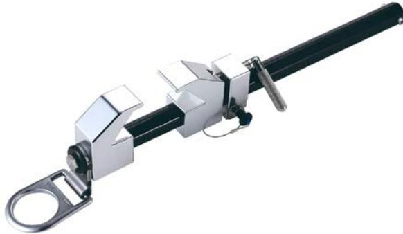
The ZERO® MultiBeam is a temporary anchorage point for both horizontal and vertical use. Designed to clamp to any beam flange and used in conjunction with a shock absorbing lanyard or a self retracting lifeline, the I MultiBeam can also be used with a positioning lanyard for work restraint.
