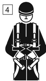
4 Connect the buckle and adjust the webbing of work positioning belt.
