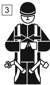
3 Connect front buckle and adjust the tension the chest strap.
