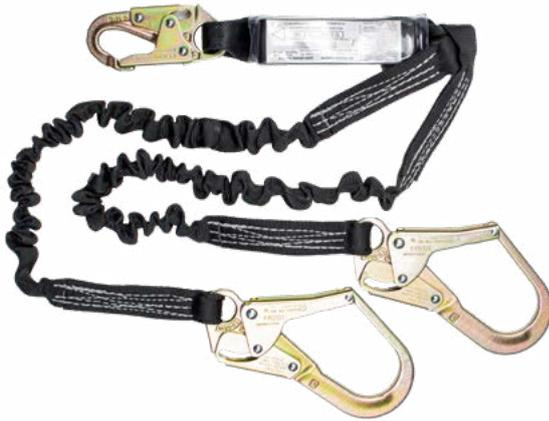
With a 181kg rating the ScaffPro X is a popular with scaffolders, construction and plant maintenance workers. The twin-tailed elasticated lanyard is designed for continuous 3-point connection to reduce the risk of a fall and the compact elasticated twin legs provide unhindered movement when not in use.
